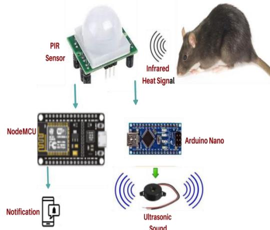
Fig (1).Overall system setup
